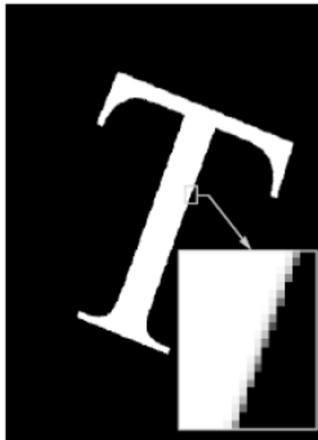
Rotation by 21° using inverse mapping and bilinear interpolation
